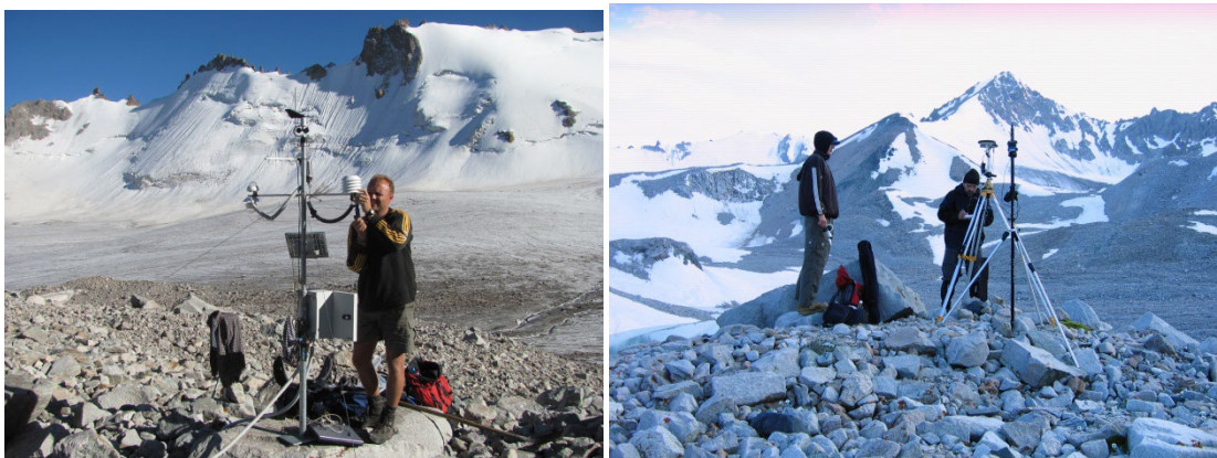
Fig. 8. Installation of automatic weather stations and GPS navigation instruments
