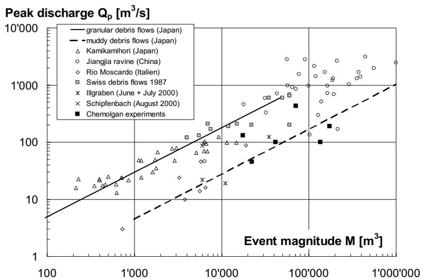
Fig. 7. Comparison of the peak debris flow discharge ( $Q_{p,DF}$ ) and event magnitude ( $M$ ). For the Chemolgan experiments, the mixture volume passing at cross-section no. 42 (values from Table 1) are used for the event magnitude.
