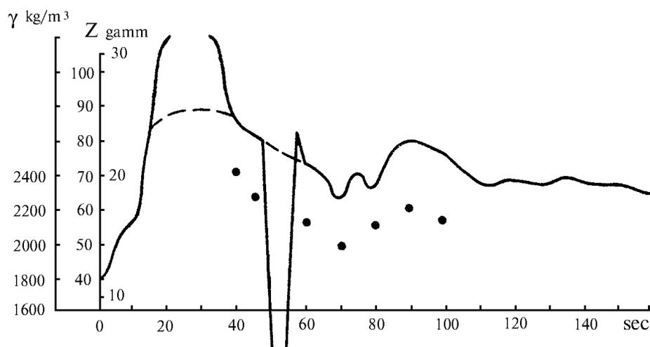
Fig. 4. Magnetic field anomaly induced by the debris flow, and values for density (shown as dots) obtained by interpretation.
