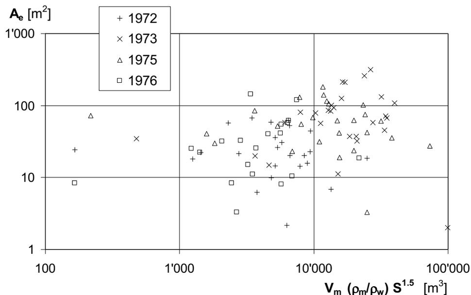
Fig. 9. Volume of eroded solid material per unit length of channel reach versus integrated "hydraulic load" of the mixture which enters the reach from upstream.
