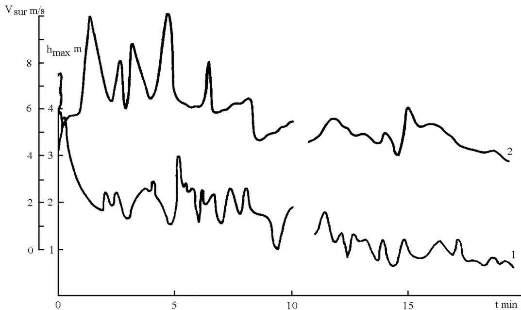
Fig. 3. Collated plots of continuous recordings during maximum depth  $h_{max}$  (1) and surface velocity  $v_{surf}$  (2) at the stationary site.
