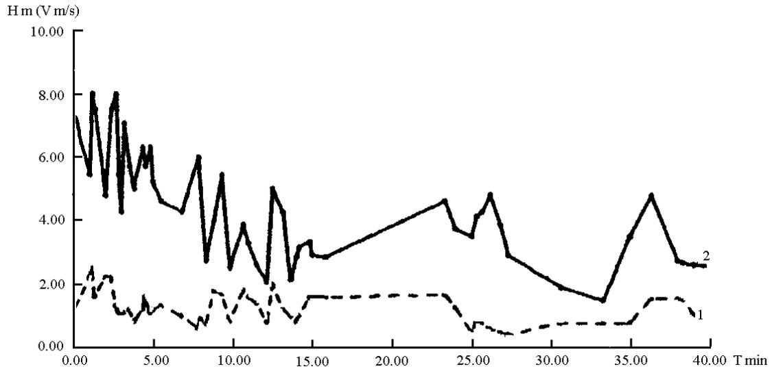
Fig. 5. An integrated plot of changes in debris-flow level (1) and velocity (2) at the control site.
