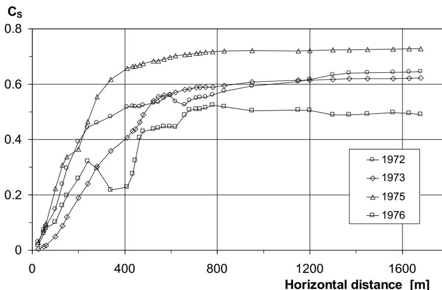
Fig. 8. Evolution of the mean solid concentration during the Chemolgan debris-flow experiments along the flow path. The bedrock reach is located at a horizontal distance from 950 m to 1680 m.
