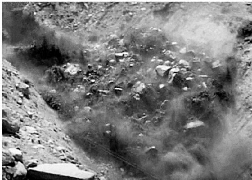
Fig. 1. Experimental debris flow in 1975 at Chemolgan test site (from Stepanov & Stepanova 1991).
