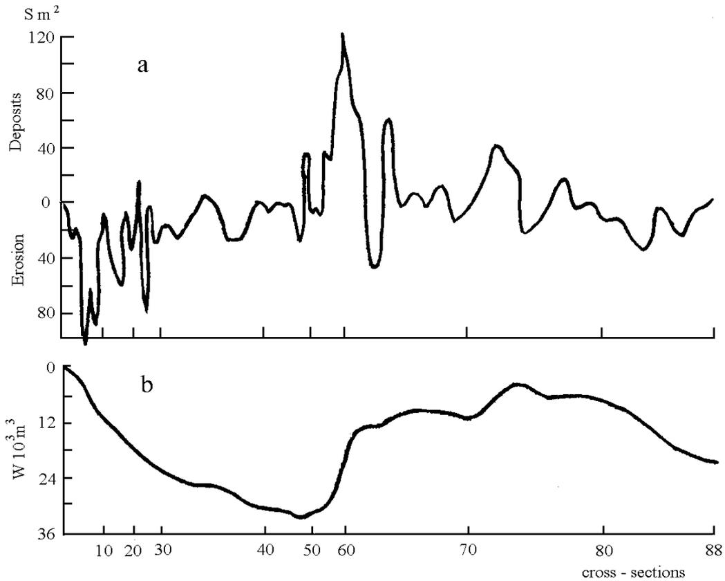
Fig. 3. Plot of areas of washout and deposits (a) according to data from levels taken of the cross-sectional profiles and an integral curve of volumes of washout and deposits (b) in 1972.
