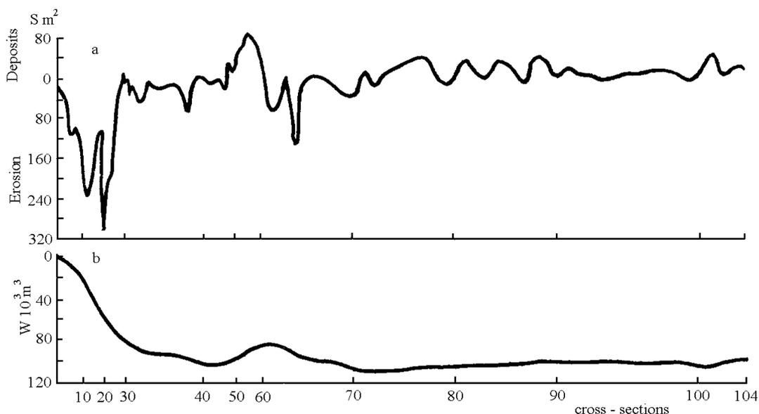
Fig. 4. Plot of areas of washout and deposits (a) according to data from levels taken of the cross-sectional profiles and curve of volumes of washout and deposits (b) in 1973.
