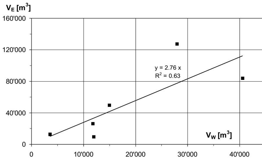
Fig. 4. Comparison of eroded soil volume  $V_E$  down to cross-section no. 42 and water volume  $V_W$  which generated the debris flows.
