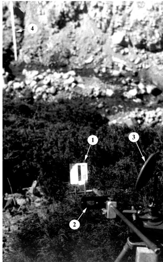
Fig. 3. Instrumentation for contactless measurement of debris-flow level.
