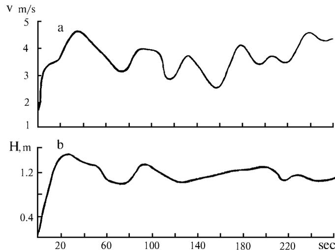
Fig. 3. Plot of the variation in debris-flow level (b) and surface velocity (a) measured at the monitoring cross section.
