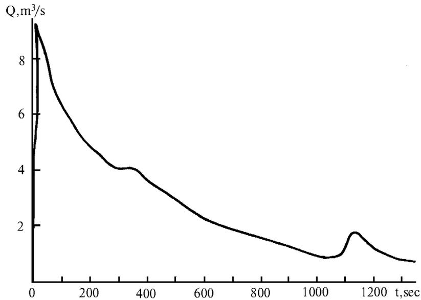
Fig. 2. Hydrograph of release from reservoir.
