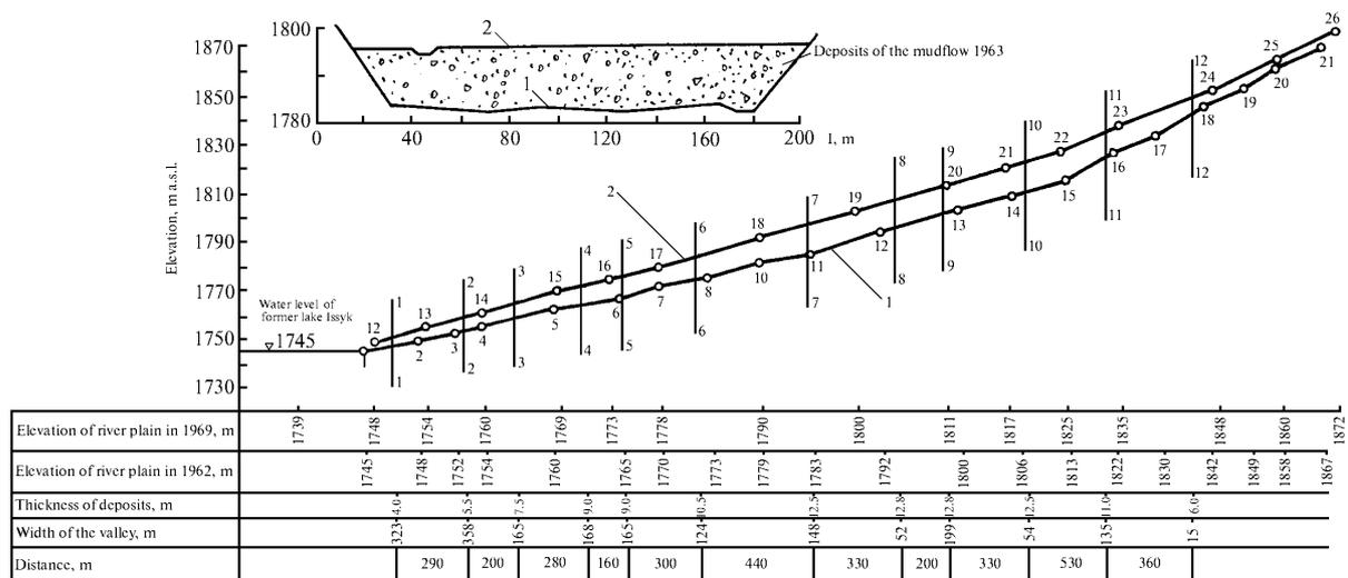
Fig. 1. Cross-sectional (cross section 7–7) and longitudinal profiles of the 3-kilometer section of the Issyk River valley above Lake Issyk.
