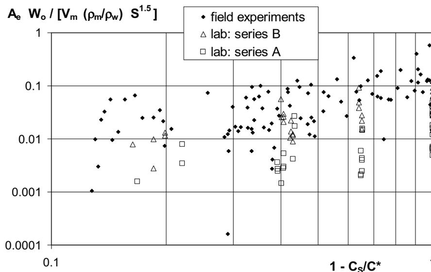
Fig. 12. The dimensionless “erosion efficiency” ratio  $B' = A_e W_o / [V_m (\rho_m/\rho_w) S^{1.5}]$  shown as a function of the expression for the solid concentration of the mixture entering the channel reach,  $(1 - C_s/C^*)$ , comparing field and laboratory data.
