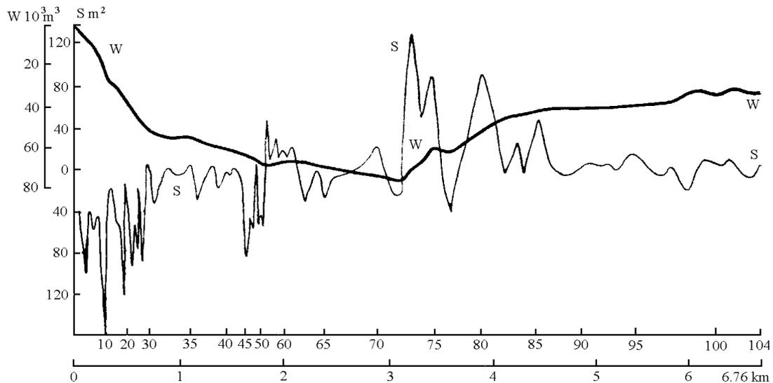
Fig. 3. Plot of areas of washout and deposits ( $S$ ) and an integral curve of volumes of removed ( $W$ ) solid material (loose).
