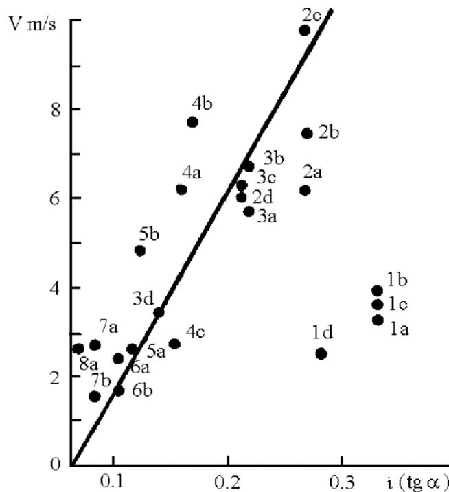
Fig. 2. The relation between velocity of debris-flow wave fronts  $v$  and channel slopes:  $a, b, c, d$  - see Fig. 1.
