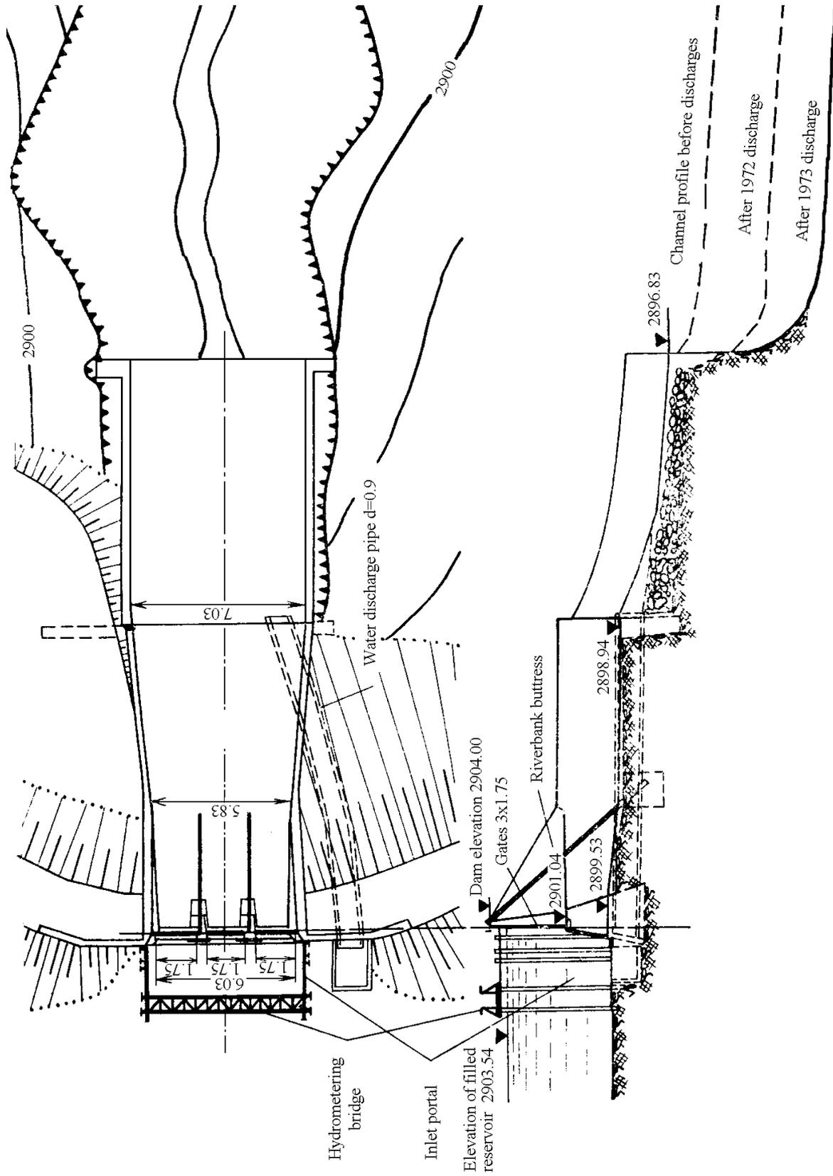
Fig. 5. Plan view and longitudinal section of dam outlet works.
