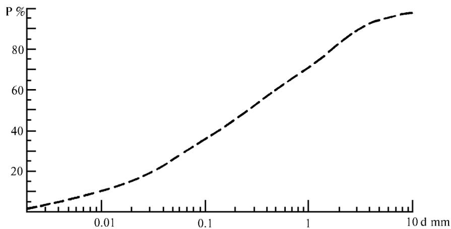
Fig. 5. Granulometric composition of deposits from the 1963 debris flow on branches of spruces left intact above Lake Issyk.
