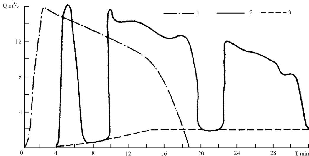
Fig. 1. Hydrographs of water releases from the reservoir in 1972 and 1973 computed according to hydraulic formulae: 1 - hydrograph of the 1972 release; 2 - hydrograph of the 1973 release; 3 – hydrograph of the release from the tubular water conduit in 1973.
