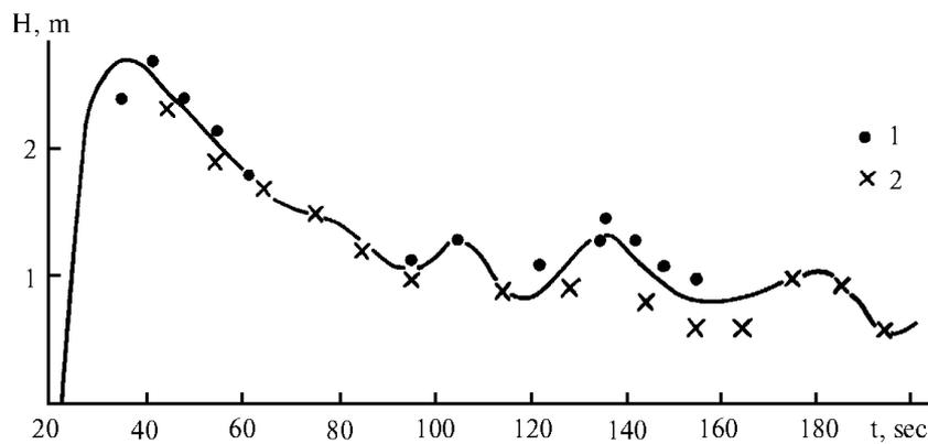
Fig. 3. Variation in debris-flow level. 1 - level gage data, 2 photo-film data.
