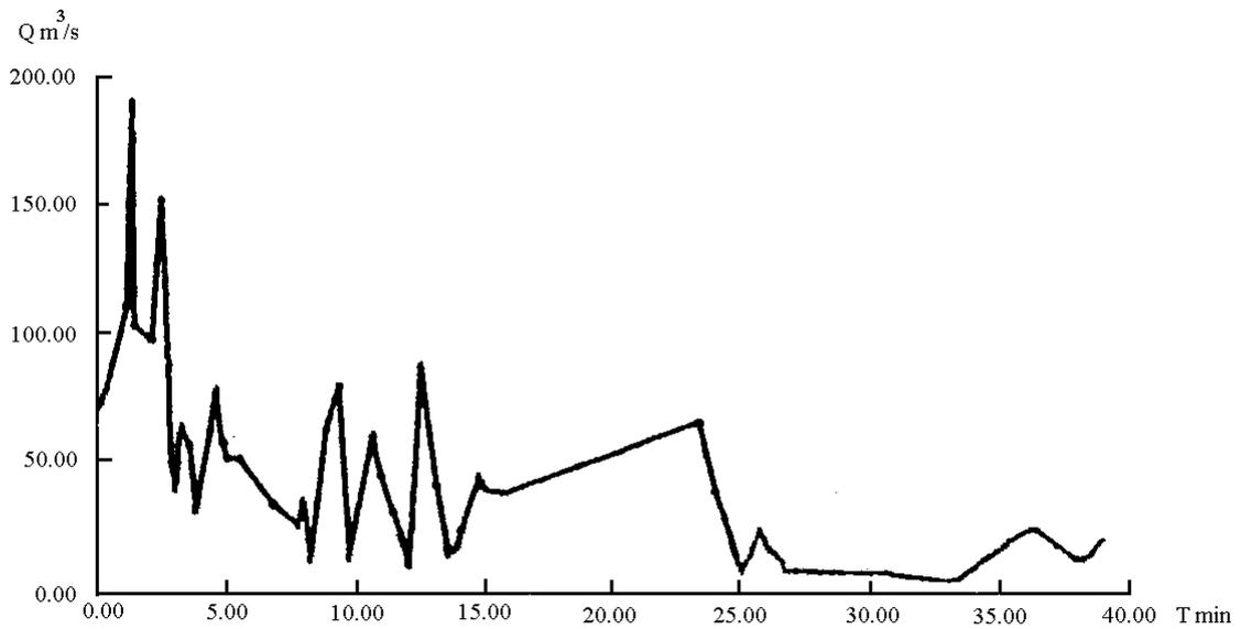
Fig. 6. Hydrograph of the debris flow at the control site computed by area and velocity.
