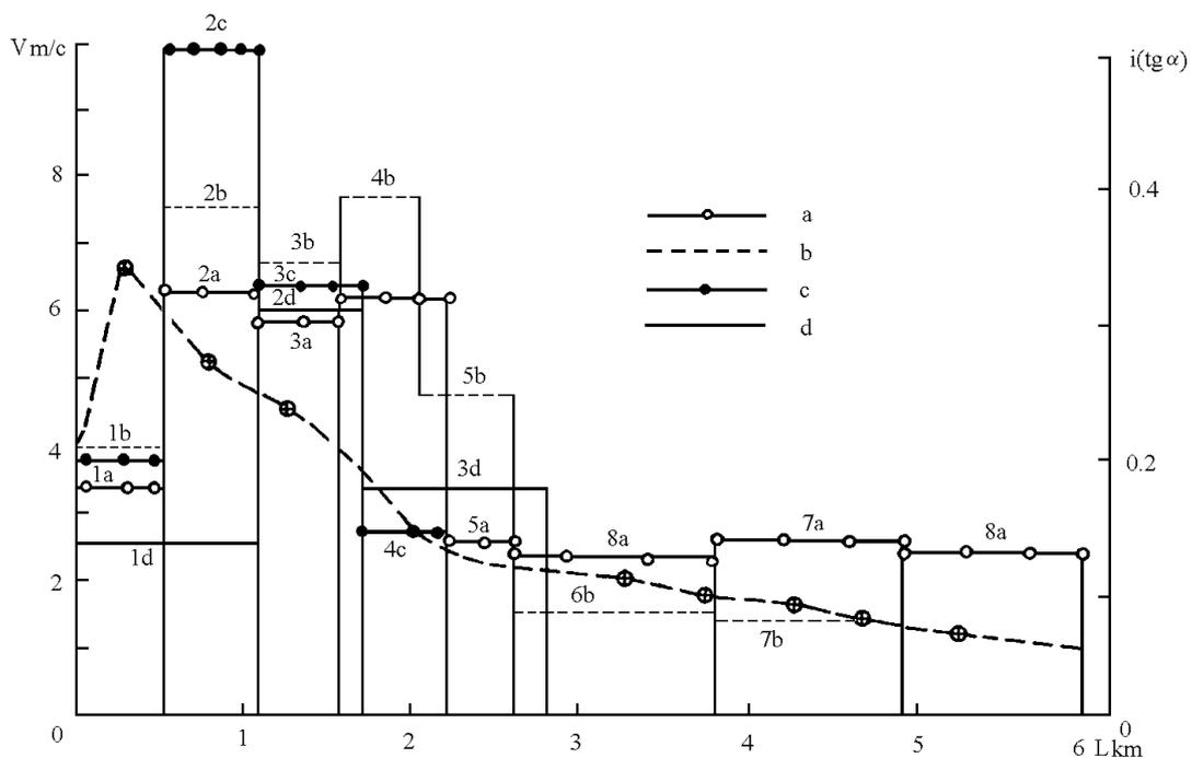
Fig. 1. Velocities at which the front of the flow  $v$  moves in various sections of the initiation zone and torrent channel:  $a, b, c$  - respectively the 1st, 2nd and 3rd waves in the 1973 experiment;  $d$  - the 1972 experiment: dotted line - slopes of the channel.
