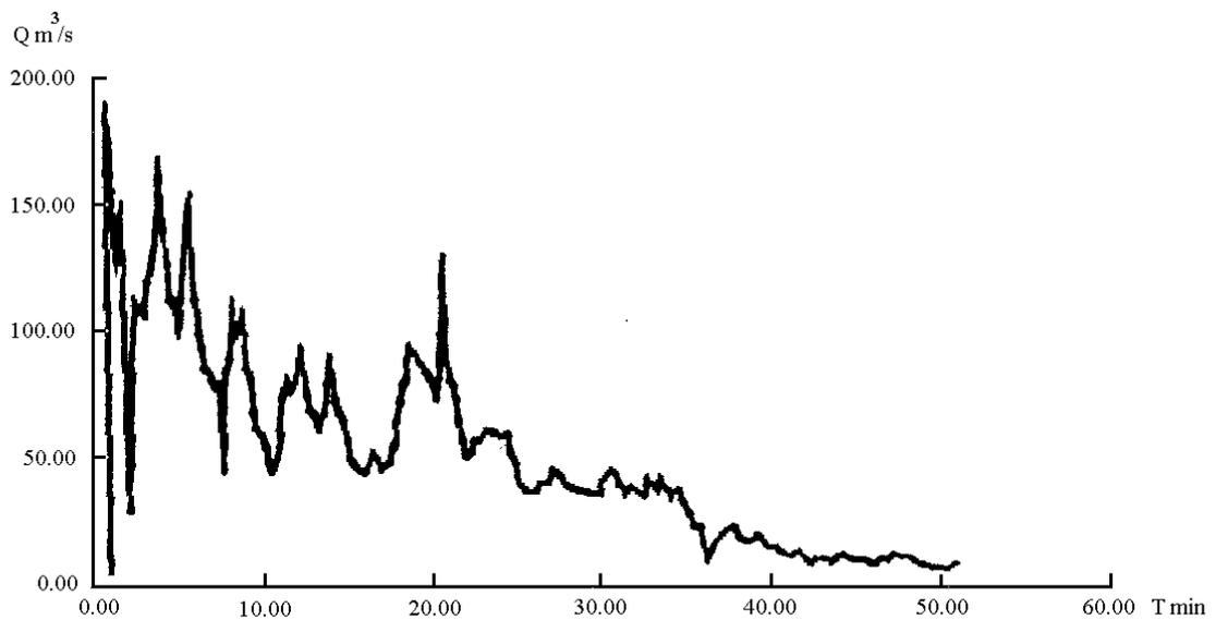
Fig. 7. Hydrograph of the debris flow at the control site (by seismic flowmeter).
