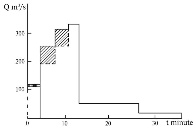
Fig. 1. Hydrograph of discharges during the outburst of lake 2.
