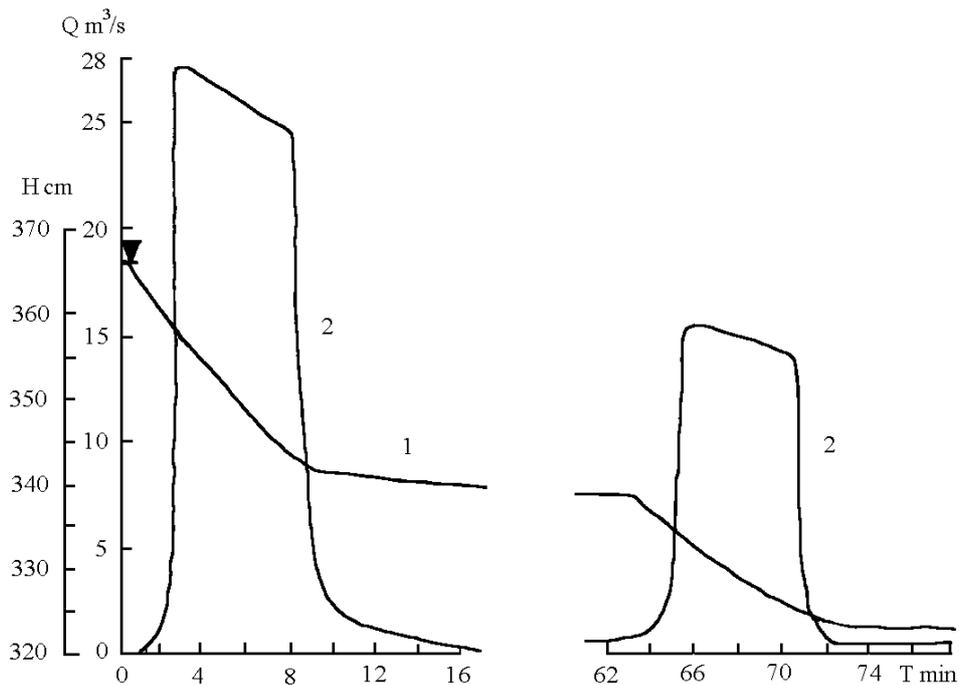
Fig. 1. Change in water level (1) and hydrograph of water releases from the reservoir (2).
