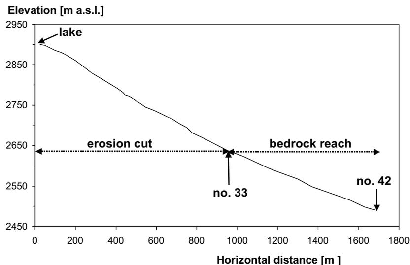
Fig. 2. Longitudinal profile of upper part of debris-flow test site at Chemolgan River.
