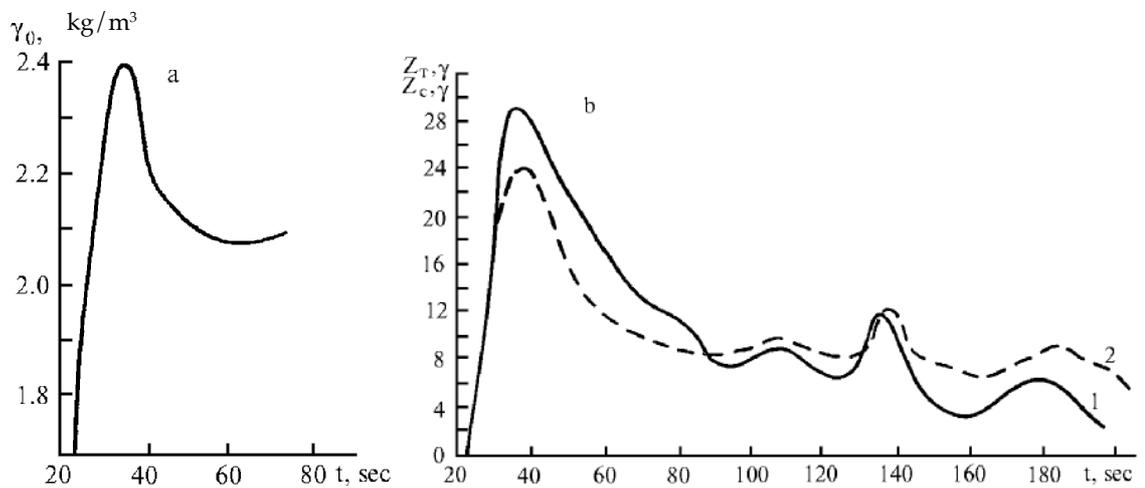
Fig. 8. Variation in debris-flow density (a) and magnetic field strength (b)
