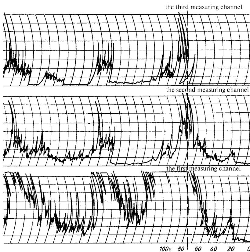
Fig. 2. Oscillograms of seismic signals produced by the debris flow.
