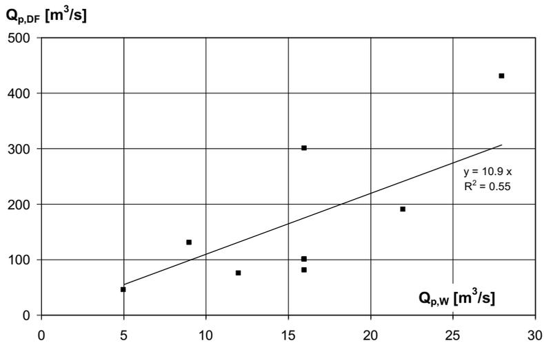
Fig. 6. Comparison of the peak debris flow discharge ( $Q_{p,DF}$ ) and the peak water discharge ( $Q_{p,W}$ ).
