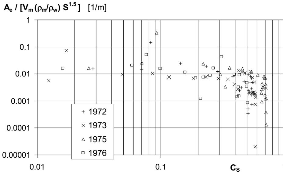
Fig. 10. The “erosion efficiency” ratio  $B = A_e / [V_m (\rho_m / \rho_w) S^{1.5}]$  shown as a function of the solid concentration of the mixture entering the channel reach,  $C_s$ .
