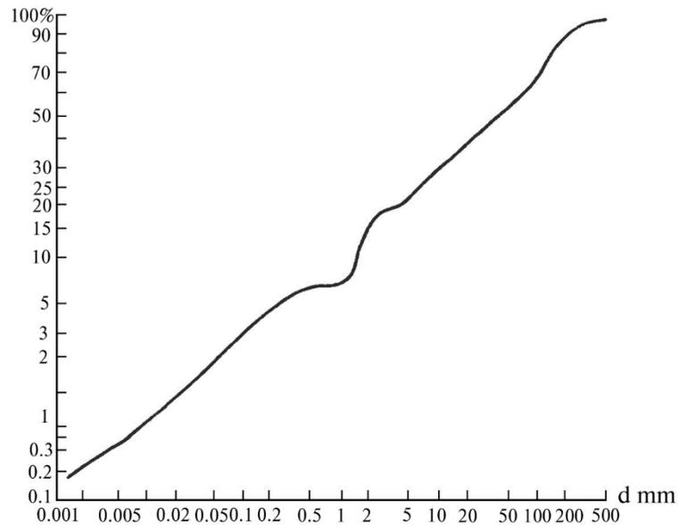
Fig. 9. Integral curve of the granulometric composition of the debris-flow forming soil of the Malaya Almatinka torrent gully.
