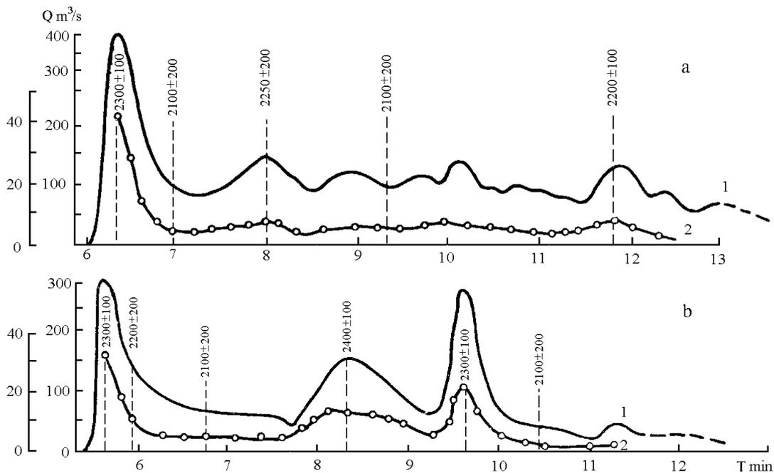
Fig. 2. Hydrograph of debris flow (1), change in magnetic field intensity with time (gamma) (2):
