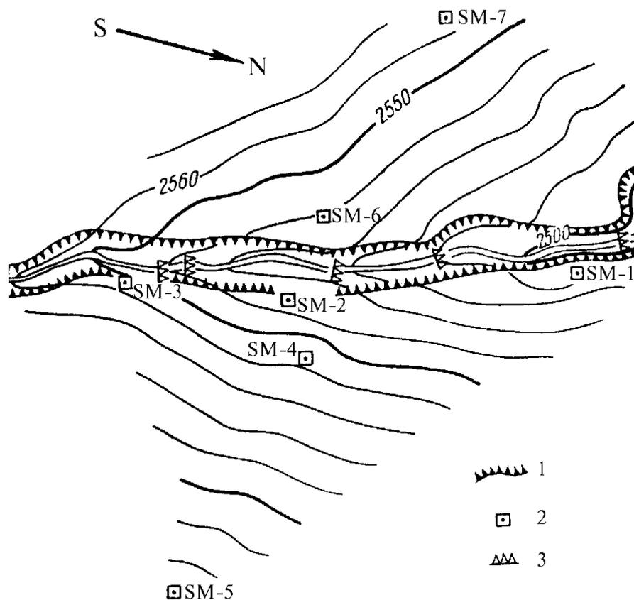
Fig. 3. Placement of seismic transducers of the warning system in the 1976 experiment: 1 - escarpment, 2 - seismic transducer, 3 - waterfall.
