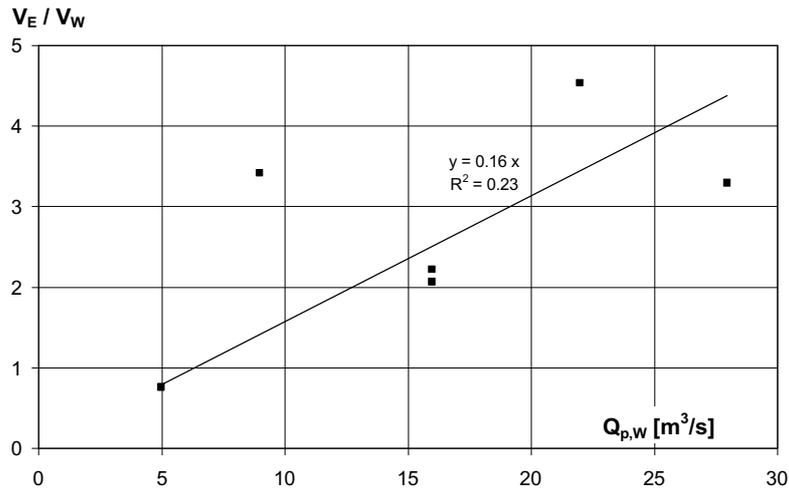
Fig. 5. Comparison of the mean ratio of eroded soil volume ( $V_E$ ) to water volume ( $V_W$ ) (down to cross-section no. 42) and peak water discharge ( $Q_{p,W}$ ).
