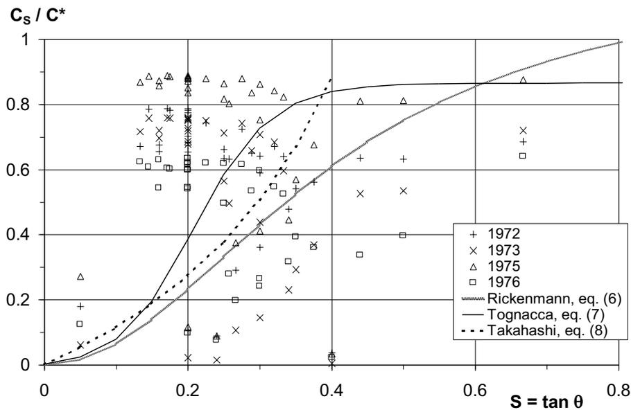
Fig. 11. Solid concentration of the mixture entering the channel reach ( $C_s$ ) vs. bed-slope of the reach ( $\tan\theta$ ), and comparison with three equations developed for bedload transport at steep slopes and debris flows.
