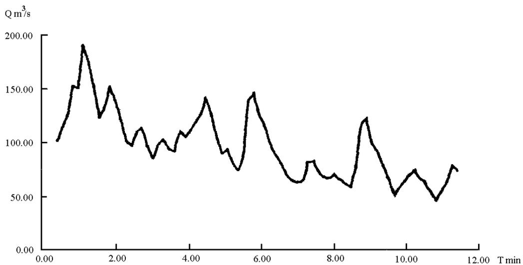
Fig. 12. Hydrograph of the debris flow at a location 100 m below the control site (from the seismic warning data).
