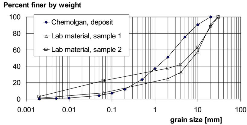
Fig. 3. Grain size distributions of material from a debris-flow deposit at the Chemolgan site and of the material used in the laboratory flume experiments.
