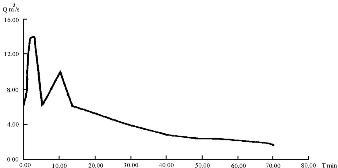
Fig. 10. Hydrograph of debris flow at the "Camp" site.
