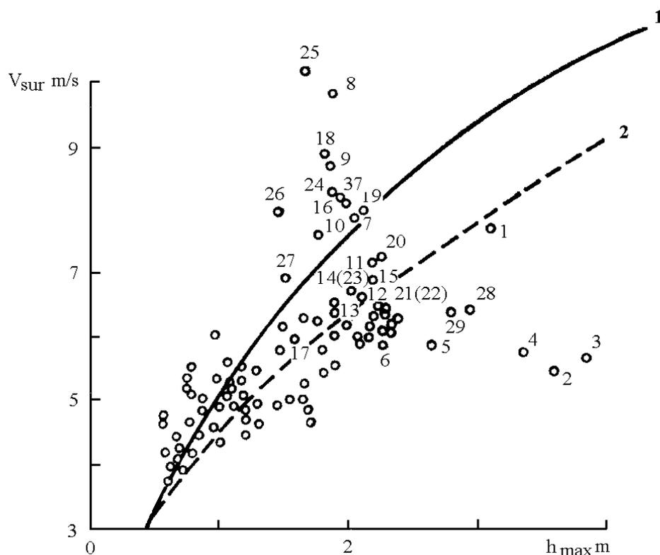
Fig. 4. Relation between surface velocity  $v_{surf}$  and maximum depth of debris flow as measured at a stationary site: 1 - based on the formula of I. I. Kherkheulidze, 2 - of V. V. Golubtsov.
