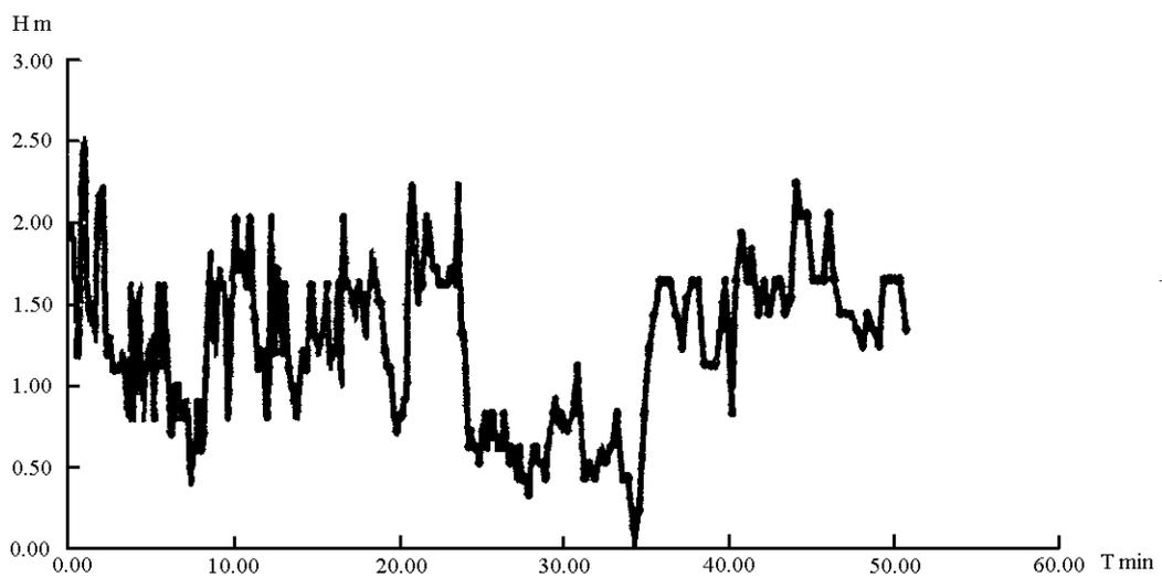
Fig. 4. Variation in debris-flow level at the control site.
