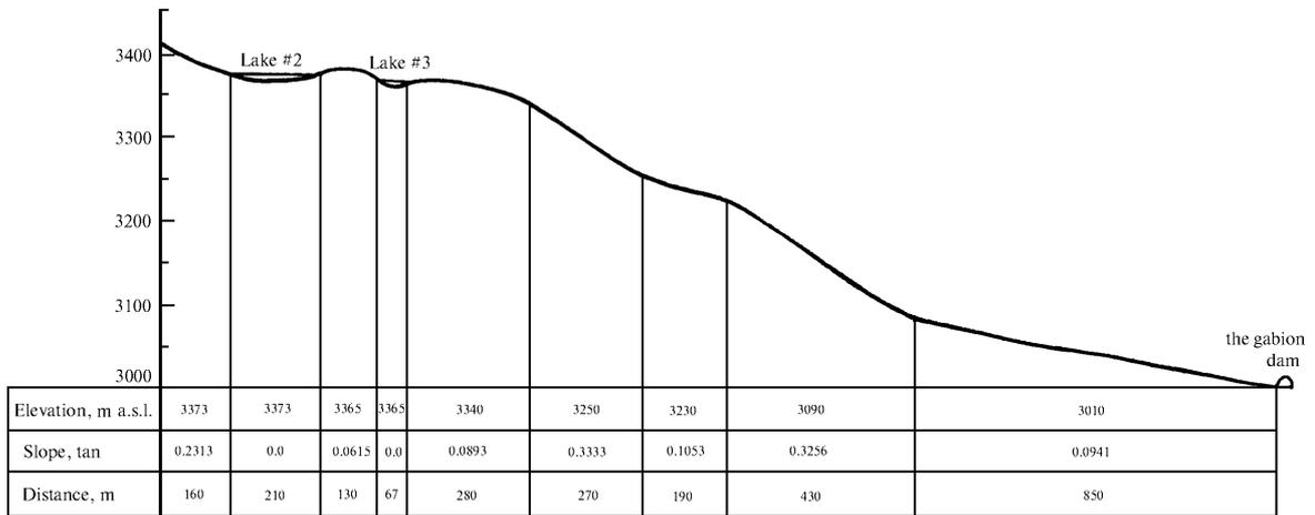
Fig. 4. Longitudinal profile of the modern moraine of the Tuyuksu glaciers in the zone of the outburst flow from lake 2 to the Mynzhilki dam.
