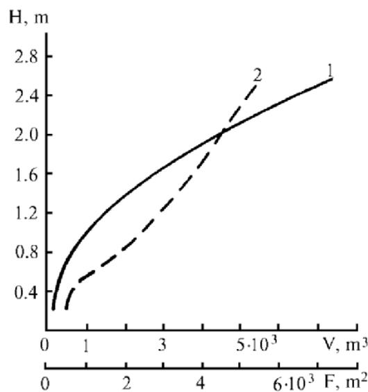
Fig. 1 Reservoir volume 1 and surface area 2 as a function of level.
