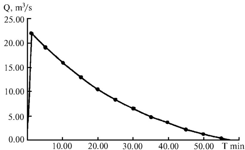
Fig. 1. Hydrograph of debris flow-forming flood.
