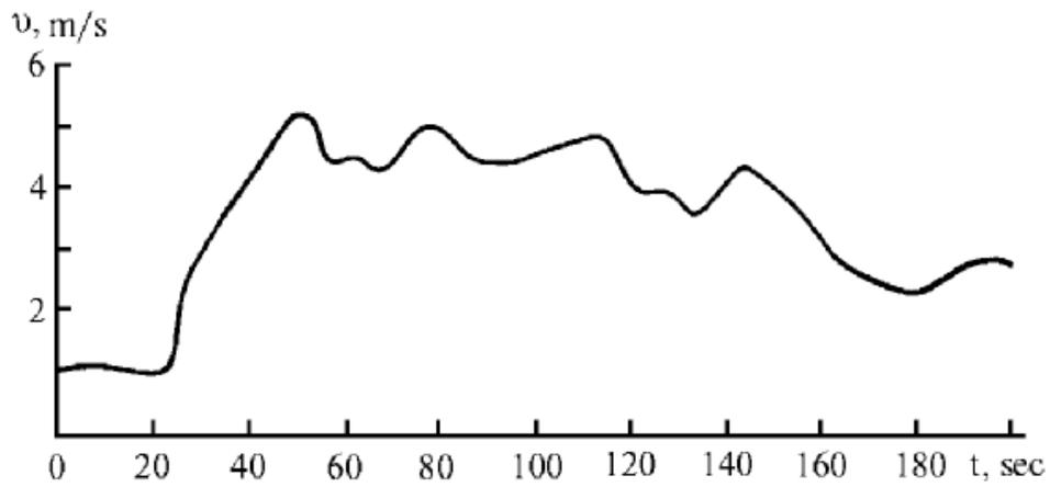
Fig. 6. Variation in debris-flow surface velocity.
