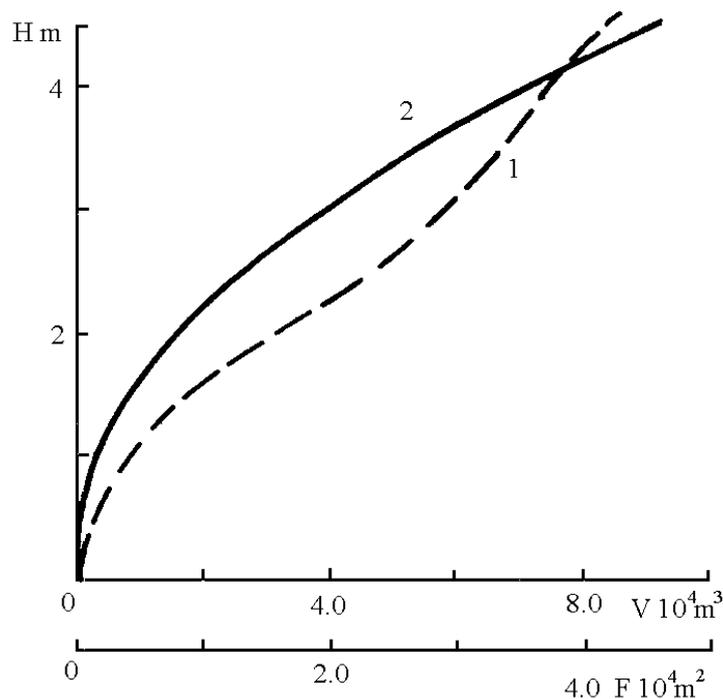
Fig. 1. Plots of the area of the water table (1) of the reservoir and its volume (2) as a function of level.
