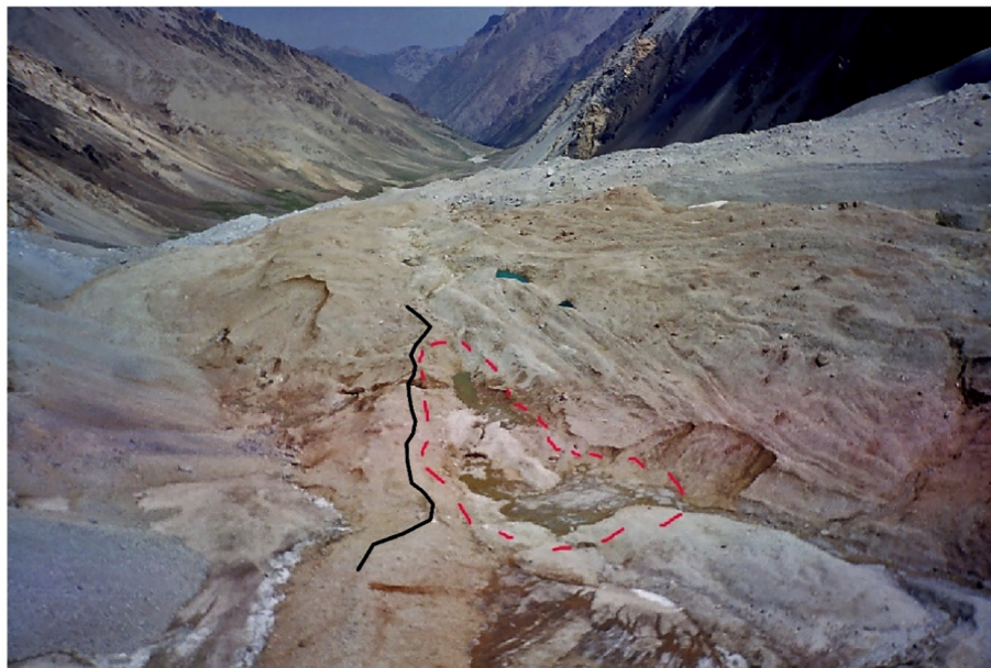
Fig. 6. Helicopter view of the initiation area of the 1998 disaster. The image was taken on August 1998. Contour of the lake is schematically shown by a red dotted line, whereas the crest of the moraine dam that was eroded during the 1998 event is given with a black line. (For interpretation of the references to colour in this figure legend, the reader is referred to the web version of this article.)
